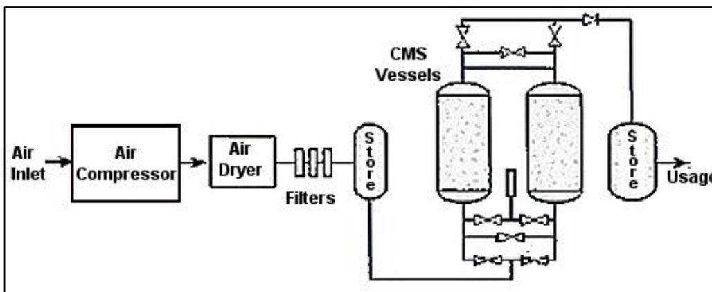
After about one minute adsorption in one adsorption tower the process controller is switching over to the second tower and the first one is regenerated.
