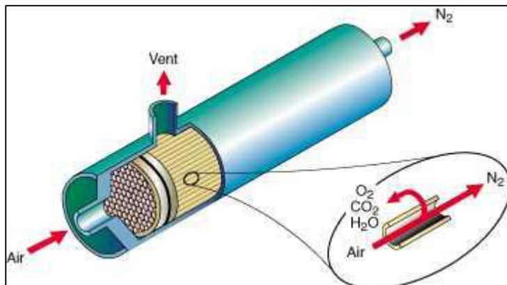
Compressed air enters one end of a permeable membrane. The membrane is comprised of many hollow fibres. The N<sub>2</sub> travels the length of the fibres and exits at the other end of the membrane. The O<sub>2</sub> in the air passes through the sidewall of the fibres and exits the side of the membrane.
